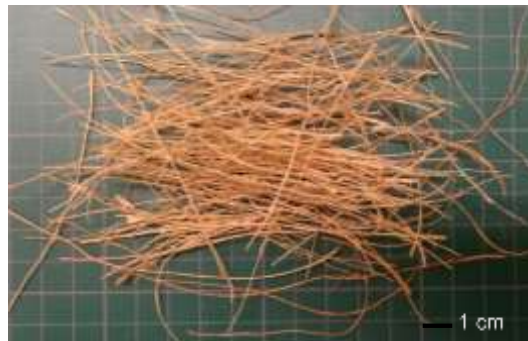
Fig. 2 Clean dry coconut fibres that were used to prepare Composite 2
