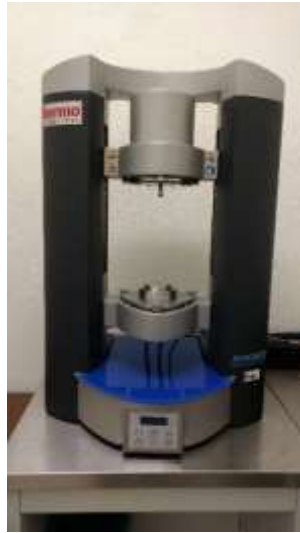
Fig. 4 Rheometer MARS III ®. Rheometer used for the viscosity and shear stress analysis of the pastes at different concentrations of microparticles.
